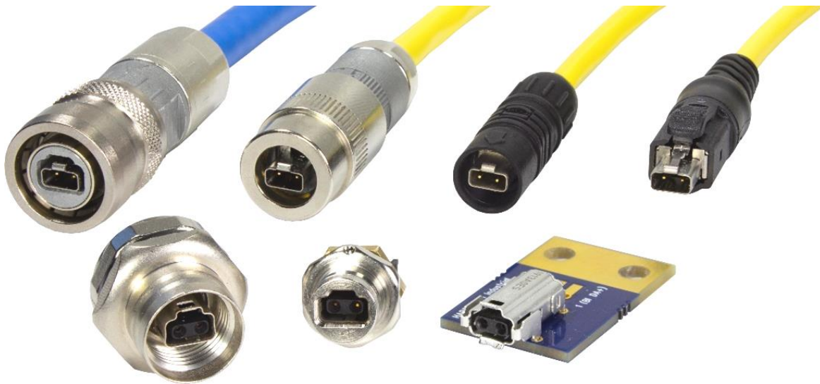
Picture 6: T1 Industrial SPE Connector versions according to IEC 63171-6 as IP65/67 as well as IP20 versions (top row from left to right: M12 PushPull Stvb., M8 PushPull Stvb., M8 SnapIn Stvb. and IP20 Stvb. / bottom row from left to right: M12 socket with screw and PushPull locking, M8 socket with SnapIn and PushPull locking, angled IP20 PCB socket) (Source: HARTING)
