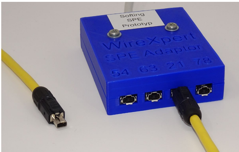
Figure 3: 4 port SP prototype adaptor for IEC 63171-6 connectivity
