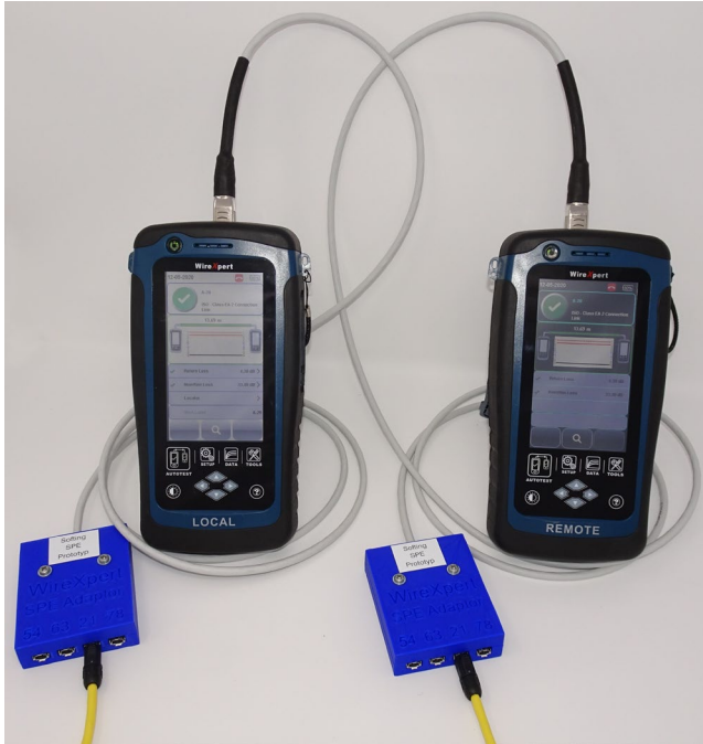
Figure 2 WireXpert 4500 with SP prototype adaptors
