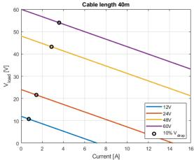
Figure 2: Voltage drop over the AWG 18 copper wire as function of transmitted power and current. (Note: The points at the curves represent the workig point with 10% voltage drop.)
