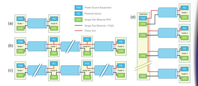
Figure 3: Network topologies hybrid connector: (a) Point to point, (b) Bus powered, (c) Bus powered with additional resupply points, (d) Switch with hybid power source
